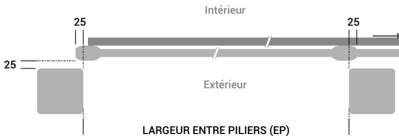
LARGEUR DE FABRICATION = LARGEUR ENTRE PILIERS (EP) + 50 MM
